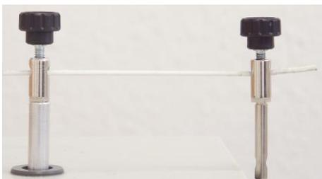
Fig. 5: Illustration of relief for transverse forces on rope.
